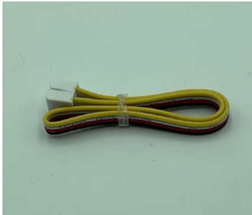
Figure 3-2. A Grove Cable
