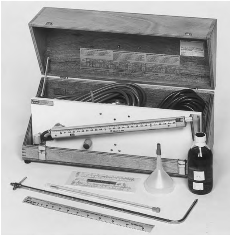
Figure 9.5 Inclined manometer. Courtesy of Airflow Development Ltd.
