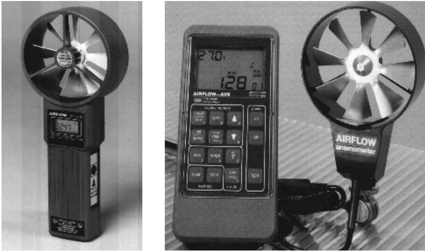
Figure 9.9 Vane anemometers. Courtesy of Airflow Development Ltd.
