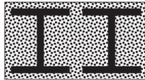
e: Multiple steel sections
